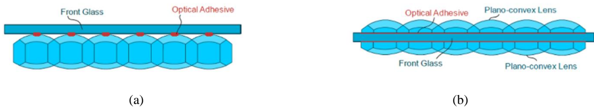
Figure 2. (a) GEN1 optical architecture (bi-convex lens mounted below glass). (b) GEN2 optical architecture (dual plano-convex lenses on either side of the front glass).
