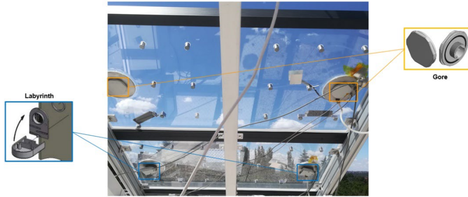
FIGURE 2. Photograph of the experimental setup consisting of two monitored mockup modules. One module uses labyrinth type breathers while the other uses Gore membrane type breathers.
