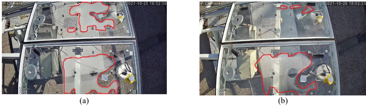
FIGURE 3. Camera view of the monitored mockup modules. Upper module contains labyrinth type breathers, lower module uses Gore membrane type breathers. (a) Condensation in both modules after adding water (b) Same modules after 3 sunny days that help de-condensation
